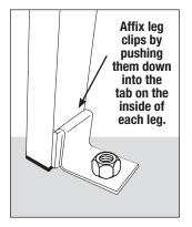
**4.** Optional: To Surface Mount, attach bench to concrete surface by clipping a leg clip (J) to the tabs on the inside of each leg. Determine your bench location and drill 4 holes into the concrete. Unscrew bolts from concrete anchors (F) and insert anchors into the holes. Position leg clips over each hole and insert bolts through the clips and into the anchors in the concrete. Tighten bolts to fully secure.
