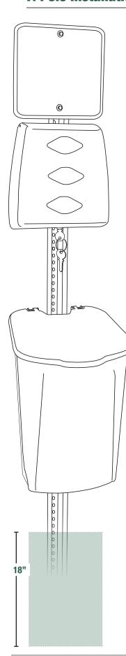
Using a post hole driver (not included), drive the sign post (C) approximately 15-18" into the ground. Make sure that the "hollow" or "recessed" side of the post is facing where you want the front of the unit to face. We recommend that the pole is no less than 15" underground to support the weight of the waste receptacle (D) properly. Use a level (not included) to ensure the pole is standing upright and will properly support the unit. Adjust if necessary.
